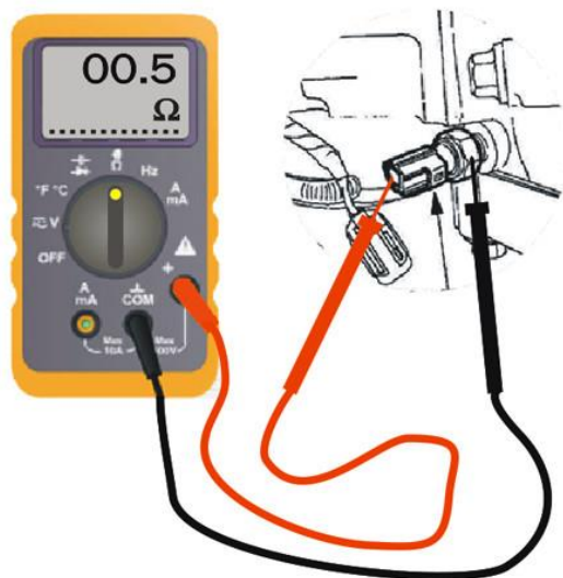
Figure 4. Multimeter probe connections for testing switch
